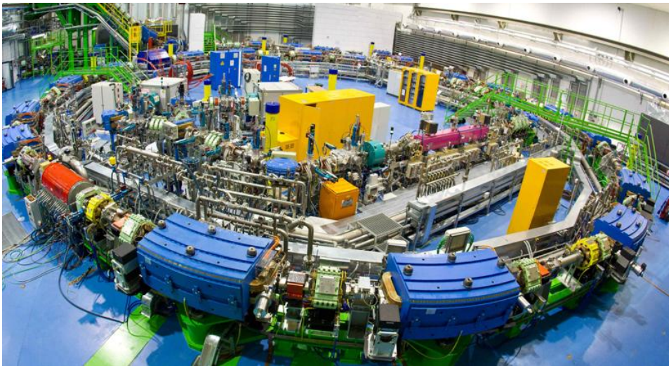
Figure 16. Picture of the synchrotron, where the heavy particles are accelerated, installed at CNAO, Pavia, Italy.
