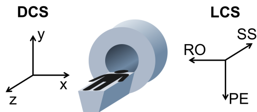
Fig. 3.10: Coordinate systems in an MRI scanner. Left: the (x, y, z) device coordinate system (DCS). Right: the (PE, RO, SS) logical coordinate system (LCS). The DCS is fixed, while the LCS depends on subject orientation and imaging parameters. The LCS shown here is for the specific case: “head-first”, “supine” with axial acquisition and A→P PE direction.
