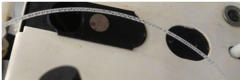
Figure 1. Air-liquid segmented flow stream.
