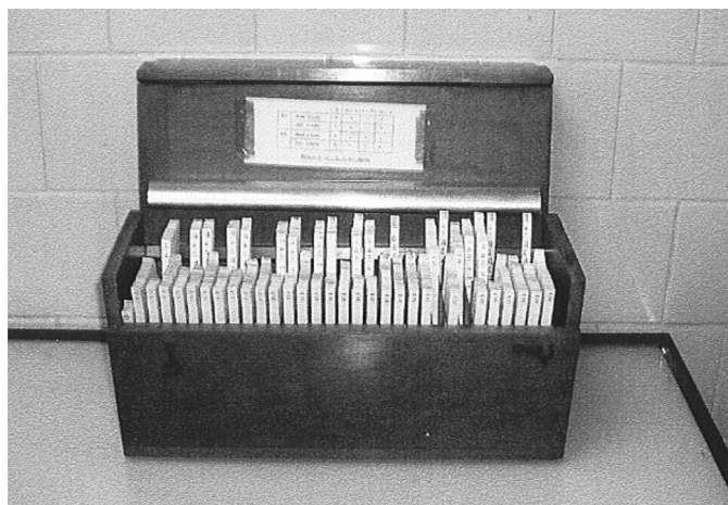
Figure 8. A set of Beavers-Lipson strips for calculating X-ray structure factors by hand, still available at the Dipartimento di Chimica in Milano. Readers who may need to use the set, because of computer breakdown, are welcome to contact the author.
