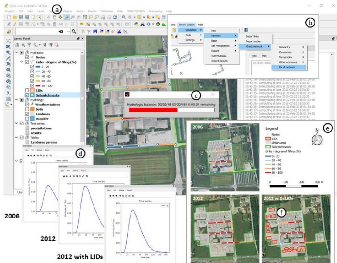
Figure 5: Mosaic of some steps in the use of the SMARTGREEN plugin: a) general GIS framework, b) SMARTGREEN menu items, c) MOBIDIC-U running, d) hydrographs for different scenario e) map of the degree of filling of the drainage network and f) particulars of LID elements.
