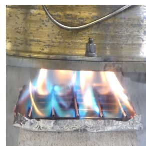
Figure 3. Cone calorimetry test.
