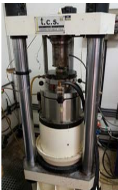
Fig. 3.11. Single stage piston – cylinder apparatus at the Laboratory of Experimental Petrology of the University of Milan (Italy).
