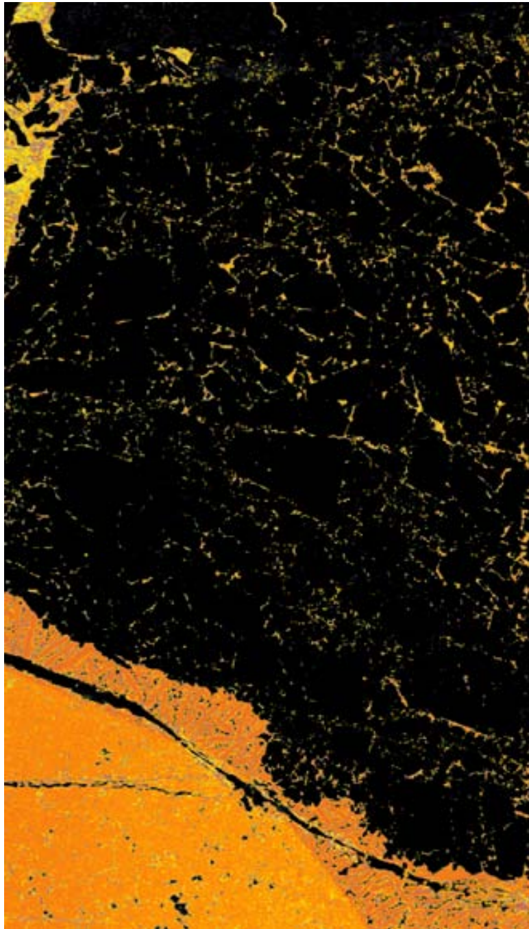
Fig. 4.38. Ca X-ray map shows in orange the carbonatitic phases, at the bottom the carbonate grains and at the interface with dunite the dendrites and into the dunite rod (black) the interconnected melt channel.
