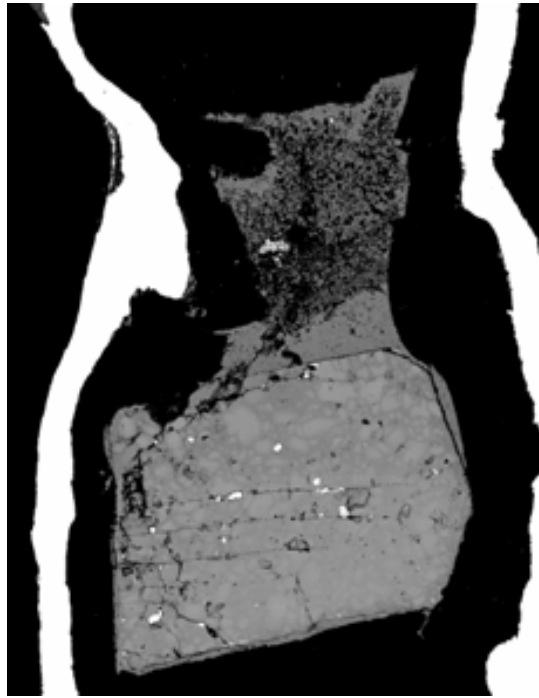
Fig. 4.17. BSE image of experimental run LSI_5 ( P = 2.5 GPa and T = 1100 °C).
