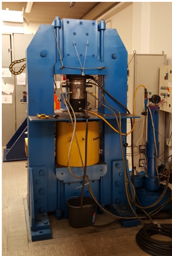
Fig. 3.13. End – Load piston cylinder apparatus at the Laboratory of Experimental Petrology of the University of Milan (Italy).
