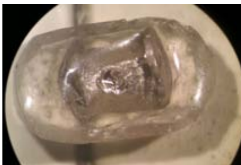
Fig. 3.25. Pierced capsule mounted in epoxy resin. Please note that the piercing technique does not affect the integrity of the capsule, allowing further investigations by means of electron microscopy and electron microprobe.
