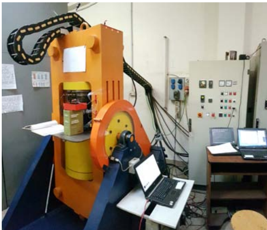
Fig. 3.16. End – Load rocking piston cylinder apparatus at the Laboratory of Experimental Petrology of the University of Milan (Italy). Orange part completes a rotation of 180 ° during runs.
