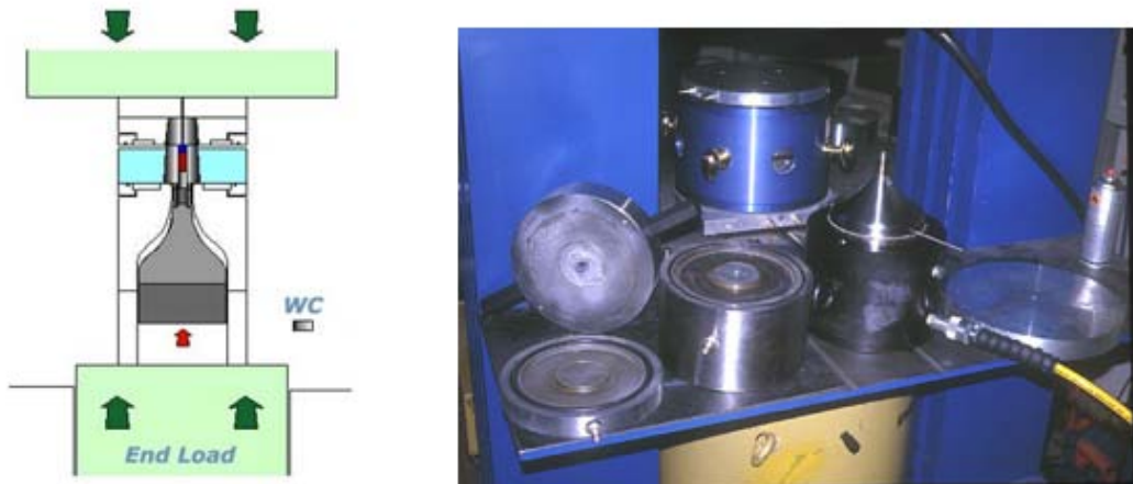
Fig. 3.14. Mechanical scheme of end – load piston cylinder apparatus on the left; parts of end – load piston cylinder with bomb and bridge on the right (Image from http://users.unimi.it/spoli/ ).
