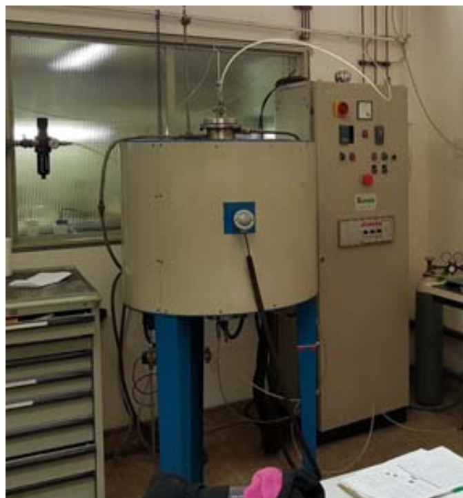
Fig. 3.7. Gas Mixing furnace used for capsule preconditioning (Laboratory of Experimental Petrology of the University of Milan (Italy)).
