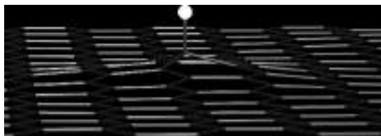
Figure 1.5: Structure of an H atom chemisorbed on graphene showing the extended puckering of the surface around the adatom.
