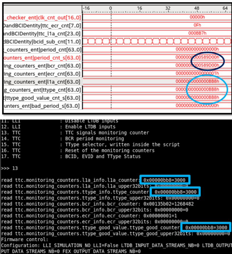
Figure 6.29: Calibration run taken with TDAQ partition: 3000 events at 40 Hz delivered. SignalTap tool (top) and firmware registers (bottom) pictures show the correct behaviour of the TTC firmware block: the number of BCRs received and BCR with good periodicity are matching (dark blue) as well as the number of L1A, TType and TType with expected value (light blue).
