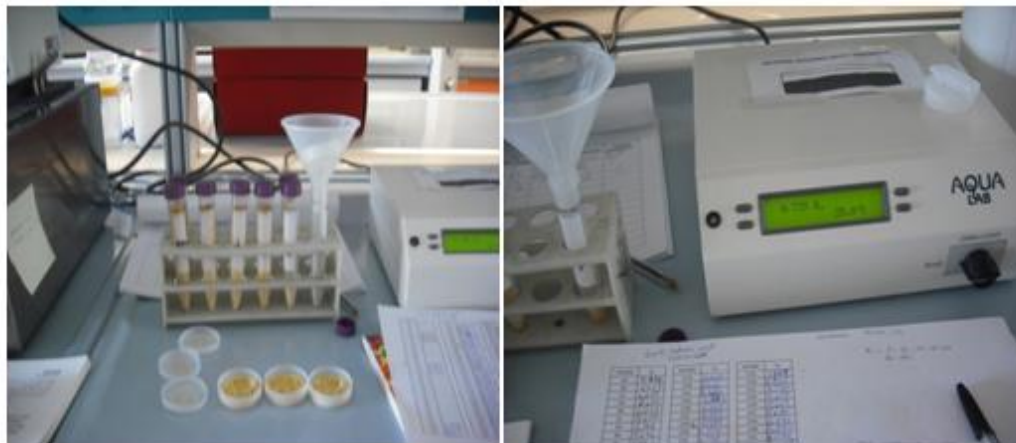
Figure 8. Sample preparation and AQUALAB CX-2 (Decagon Devices Inc., Pullman, Wa, USA) machine used for water activity tests.
