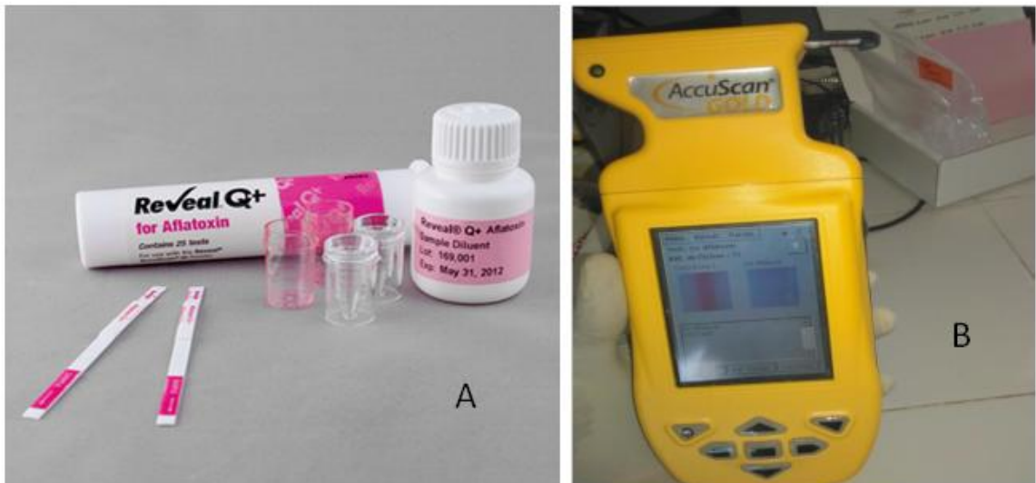
Figure 16. Aflatoxin kits (A) and AccuScan Gold detector (B) used for quantifying aflatoxin content of maize grains.
