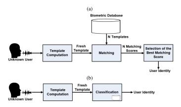
Fig. 1: Schemas of biometric identification systems: (a) systems performing multiple identity comparison, and (b) systems that search the identity of the user by classifying a single biometric template.
