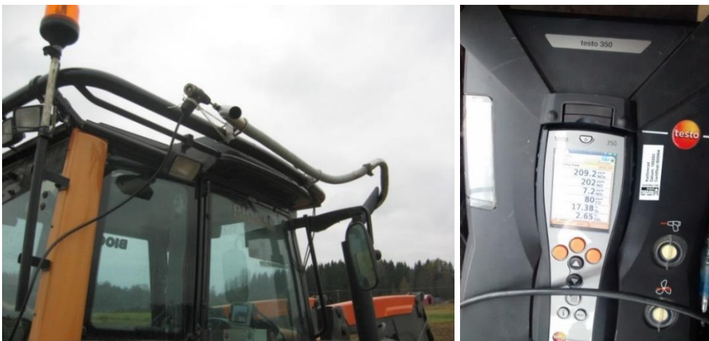
Figure 11. Part of Valtra N101 with the implemented sampling probe to collect exhaust gases and Testo® 350 on board. [Source: pictures by H. Harvidsson and D. Lovarelli]
