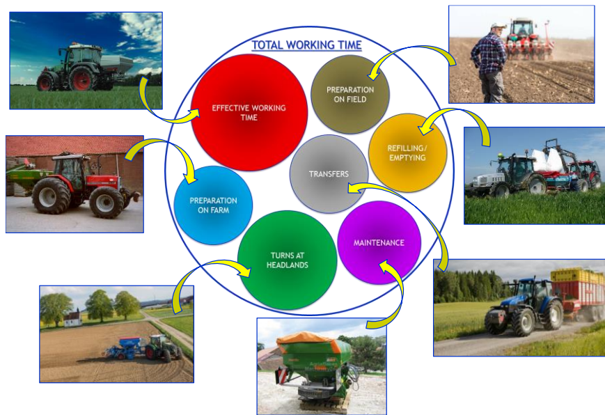
Figure 6. Total working time split in single working timings. In general terms, the dimension of the single circles is related to the relevance of those working timings along the whole operation.
