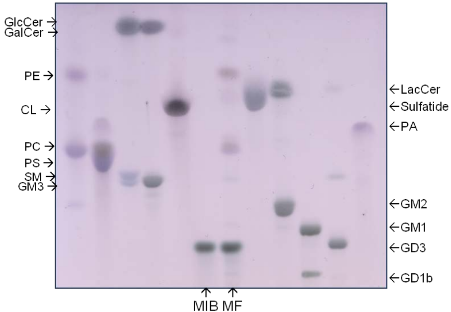
Figure 17. TLC analysis before microdialysis of total lipid extracts from isolated mitochondria (mitochondria isolated from a healthy subject of 50 y.o.). MF and MIB were subjected to lipid extraction with \text{CHCl}_3/\text{CH}_3\text{OH}/\text{H}_2\text{O} 20:10:1 (v/v/v) and loaded (40 \mu\text{g} of protein) on a silica gel TLC plate. HPTLC was performed using chloroform/methanol/0.2% calcium chloride 60:35:8 (v/v/v) as solvent system. The lipids were then revealed using anisaldehyde as colorimetric detection.
