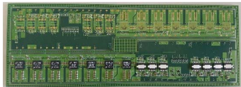
LVPS (installed near PP2, V_{out} = 24 - 48\text{ V} )
