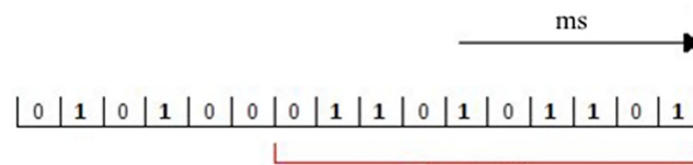
Fig 4. Light window. Each cell represents one millisecond, and the value in the cell represents the number of photons that reach the retina within the same millisecond.
