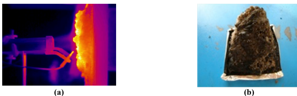
Figure 1. a) infrared image of the development of an intumescent coating at the jet fire test (propane burner, heat flux of 200 kW/m 2 ) protecting composite and b) cone calorimeter residue (experiment done at 50 kW/m 2 ) of an intumescent glass fiber reinforced polybutylene terephthalate (PBT).
