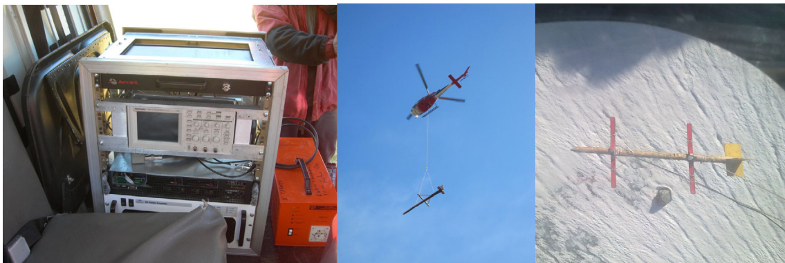
Figure 3. RES system and antenna arrangements for helicopter survey.
