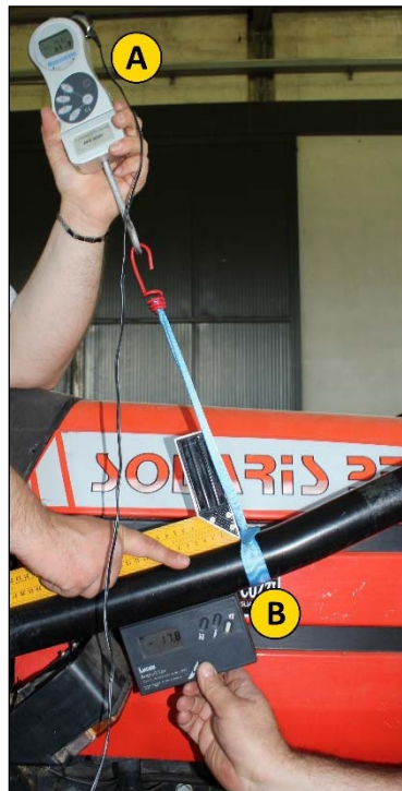
Figure 6. Static raising test (A = integrated load cell with digital display; B = digital inclinometer).
