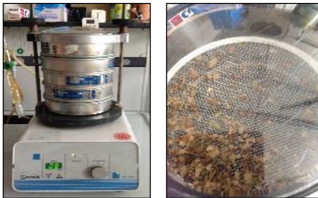
Figure 9: Vibroscreen used after seed collection in order to separate seeds from capsulaes.
