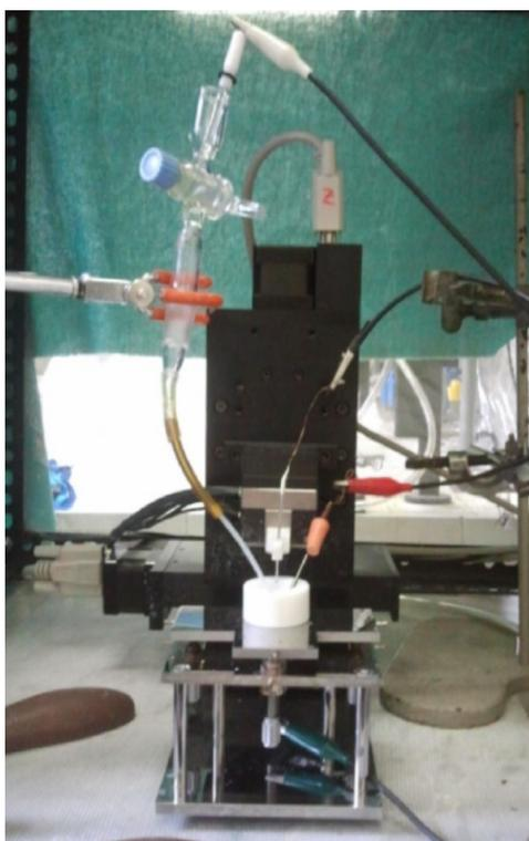
*Figure 19: Picture of a SECM apparatus.*
