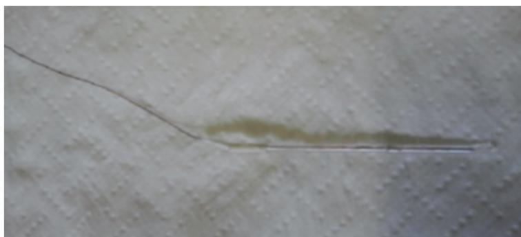
*Figure 30: Picture of an Au UME tip.*
