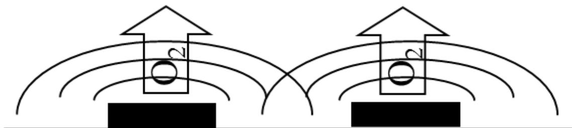
**Figure 35:** Overlapping of oxygen diffusion profiles of different spots, when they are all biased at an  $E_{OER}$  at the same time [1].
