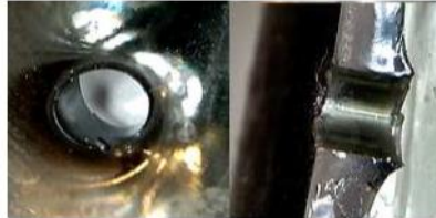
Figure 4: Top side view and section of the PDMS vias metallized by SCBI.
