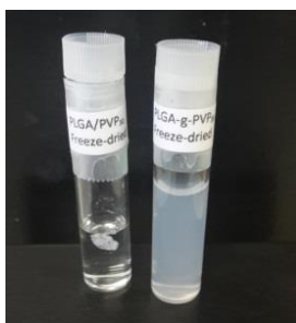
Figure 2.18. PLGA/PVP 10:3 blend and PLGA-g-PVP 10:3 MP sample re-dispersed in water after lyophilization of the pristine nanodispersions.
