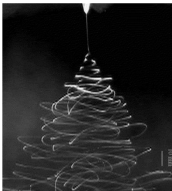
Figure 2. Particular of Taylor cone and helicoidally motion of fibre jet. Figure take from reference. xvi
