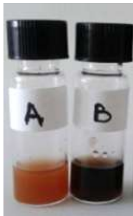
Fig 15. Water dispersions of MEEA- (A) and ZDS-coated (B) iron oxide NPs. Image from Ref 21.
