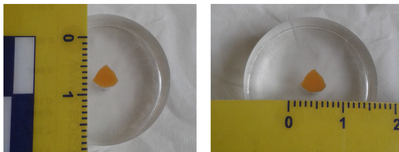
Figure 3.3: Polished BaTi_{0.8}Ce_{0.2}O_3 ceramic sample, not yet coated, prepared for electron microprobe analysis. Centimeter scale.
