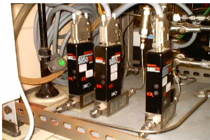
Figure 4.4: Volumetric flowmeters for the regulation of CO, H 2 and N 2 flow.
