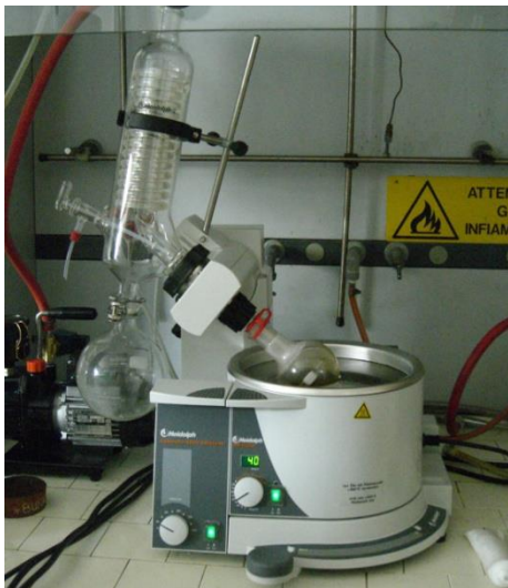
Figure 5.1: Rotary evaporator used for the synthesis of Fe 30 K 2 Cu 3.75 .
