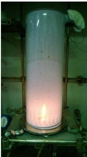
Figure 5.3: Pyrex manifold during the FSP synthesis.
