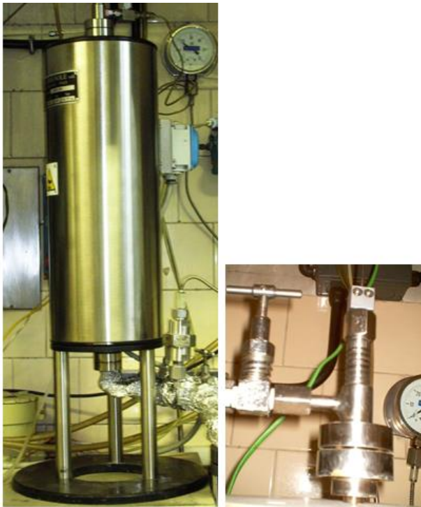
Figure 4.5: FT tubular reactor (left) and upper flange (right).
