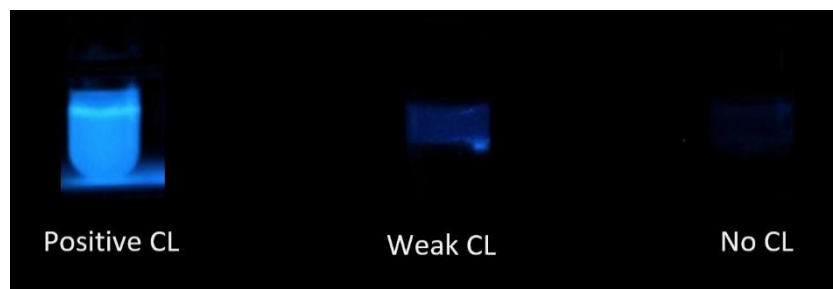
Fig. 2.4 - different degree of chemiluminescence intensities produced by different amount of Hb preserved in bone powder.
