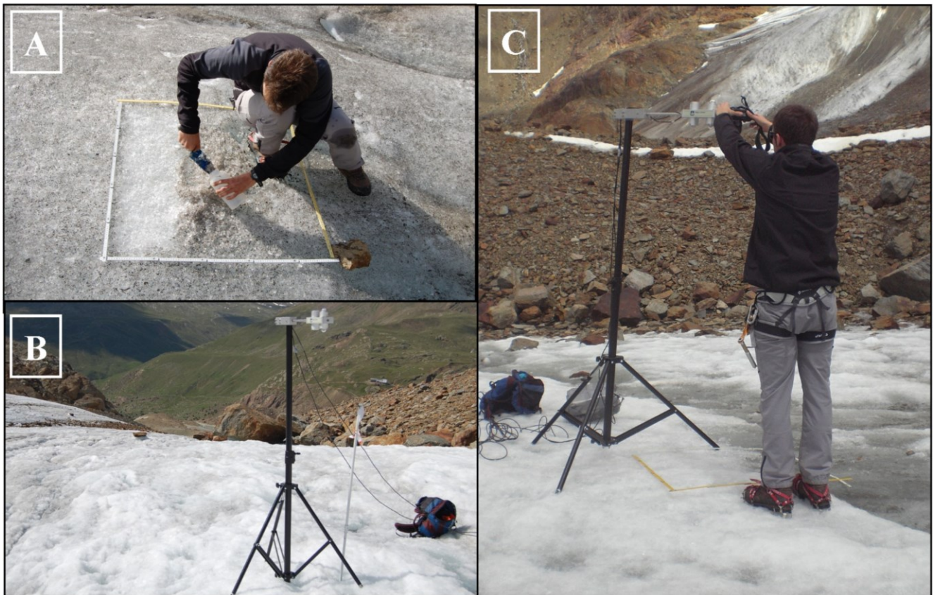
Fig. 2: Series of pictures illustrating: (A) sampling supraglacial debris, (B) measuring albedo and (C) acquiring high-resolution digital images of the glacier surface.
