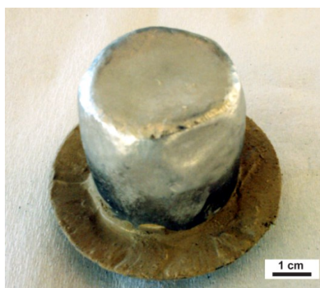
Figure 4.1: Platinum crucible configuration during the laboratory furnace thermal treatments.
