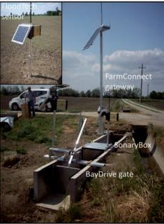
Figure 2. Design and installation of the bay-drive gate and water level sensor in the field.
