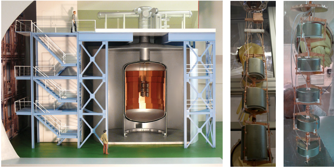
Fig. 2: Left: a mock-up of GERDA, with the water tank, the cryostat and, in the center, the detectors (not in scale). Middle: a string with three coaxial detectors prior to the installation in GERDA. Right: the first five BEGe detectors being installed in GERDA during Phase I data acquisition.
