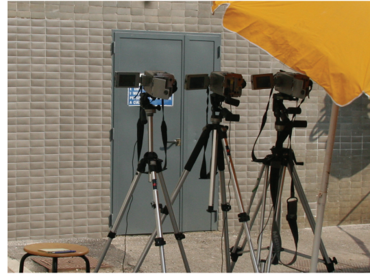
FIGURE 5: Experimental setup, three infrared camera, mod. TVS 700.
