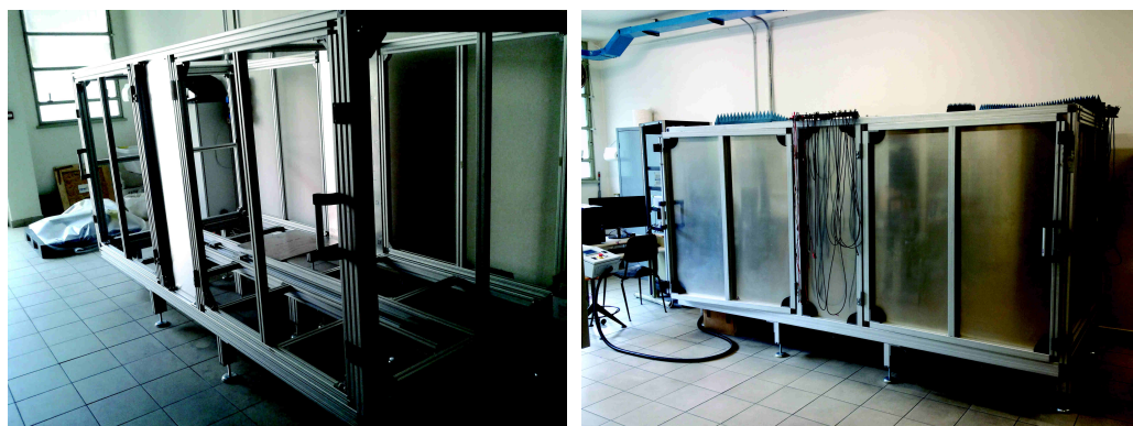
Figure 4.19: Left: the anechoic chamber in a primordial stage: the mechanical frame, made with aluminum profile system, is visible. Right: the facility is completed with the metallic shielding.
