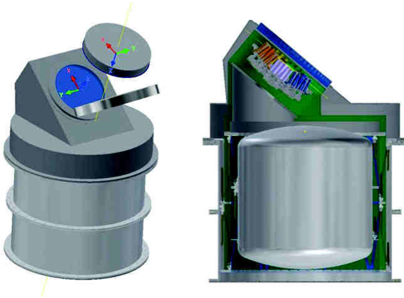
Figure 3.7: A sketch of the STRIP cryostat. Left: a view of the instrument cryostat with the footprint of the double mirror telescope. Right: the sketch shows a cut in which the focal plane array is faced to the dielectric window. The 500 liters tank contains liquid Helium for the instrument cryogenic operation at 20 K (Bersanelli et al. 2012).
