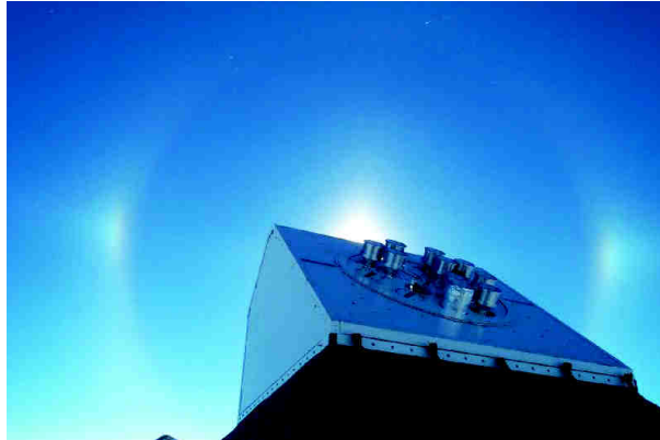
Figure 2.3: The Degree Angular Scale Interferometer, DASI. The design of the array configuration was optimized to provide continuous coverage from the minimum to maximum baseline. The minimum baseline of 25 cm, which sets the maximum angular scale, was chosen to provide coverage of the first acoustic peak in the CMB power spectrum. The maximum baseline 115 cm was chosen to overlap with the largest angular scales of the CBI experiment. To improve the (u, v) coverage and to provide redundancy checks, the entire array could be rotated along the line of sight (Leitch et al. 2002).
