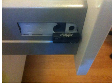
(a) Magnetic sensor attached to a drawer
