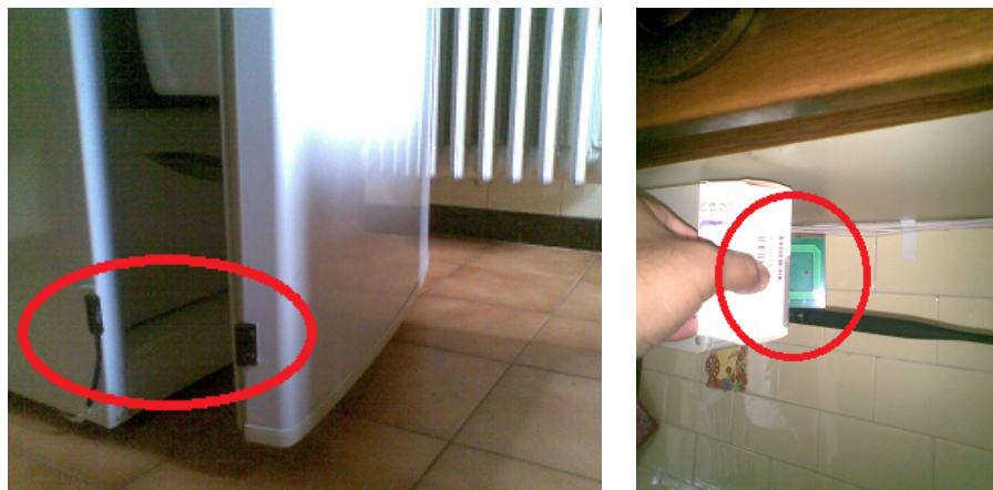
(a) Magnetic contact sensor on the fridge door (b) Passing a tagged medicine box over the RFID reader
