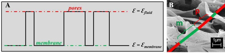
Figure 3.7: Step function of the dielectric constant inside a porous membrane along a straight line that transects the material.
