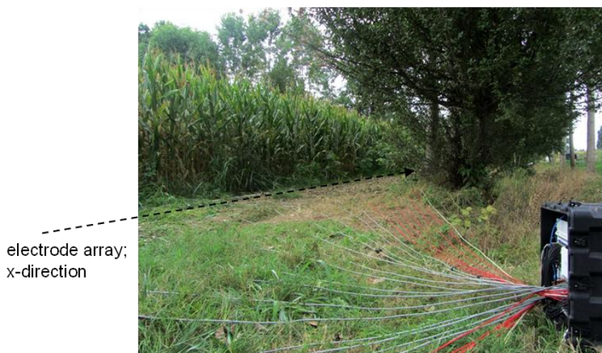
Fig. 7.26 - EIT acquisition in Landriano; the electrode array is arranged along a N60E profile.
