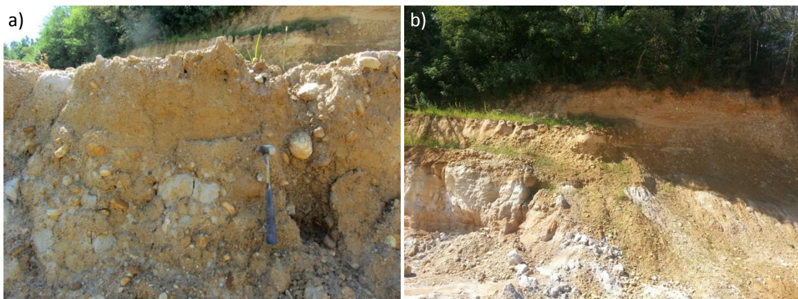
Fig. 7.39 - Silty-sand with lithic and partially consolidated pebbles of muddy-sand rich in micas ( Volpina? ) outcropping on the front wall of the quarry terrace between x = 20 m and x = 29 m (a); white lens of muddy sand ( Caolino? ) outcropping on the front wall of the upper terrace.
