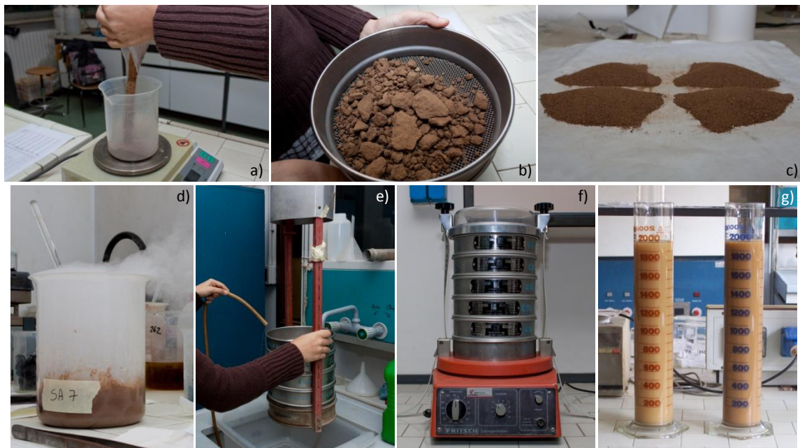
Fig. 3.9 - Phases of particle-size-distribution analysis: weighting (a), separation of the gravel fraction (b), quartering (c), oxidation of organic matter (d); humid sieving (e), dry sieving (f), and densimeter test (g).
