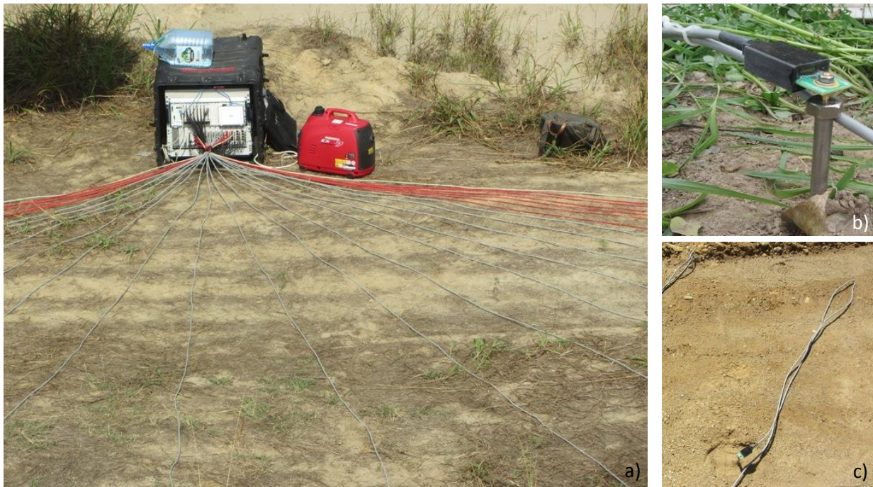
Fig. 7.24 - Radial and symmetric distribution of connecting cables between the EIT system and the electrodes (a); detail of an electrode and the corresponding amplifier unit (b); closed cable loop beyond the electrode position (c).
