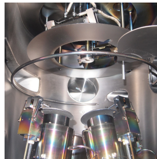
Figure A.1: (a) Schematic of a generic sputtering equipment. (b) The internal part of the Kurt J. Lesker PVD75. Two of the four confocal target sources are visible in the lower part of the picture. Above, the ring-shaped anode and the sample holder in its center.
