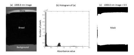
Figure 2. Masking the background from a hyperspectral image: (a) shows a single wavelength image at 1008.8 nm, (b) is a histogram showing the distribution of pixel values in (a) and (c) is a thresholded image, obtained by setting to zero all pixels in (a) that are greater than 0.5. The mask in (c) represents the sample of interest.
