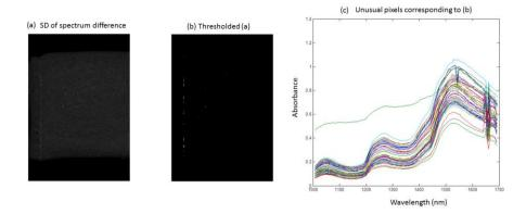
Figure 4. Identification of dead pixels. Standard deviation (SD) of difference hypercube shown in (a); thresholding (a) locates the dead pixels in (b); spectra corresponding to dead pixels shown in (c).
