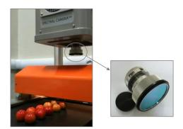
Figure 2: SisuChema NIR Spectral Camera during the acquisition of acerola samples and a detail of the 50 mm lens.
