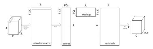
Figure 5. Application of PCA to a single hypercube extracting sample spectra from hypercube to make 2 dimensional data matrix, followed by matrix decomposition by PCA application of PCA loadings to original hypercube by unfolding, followed by re-folding to make PC scores cube.
