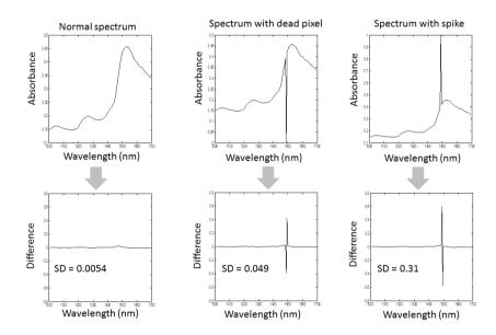
Figure 3. Normal, dead pixel and spike absorbance spectra (top row), with difference spectra and their standard deviations (SD) shown (bottom row).
