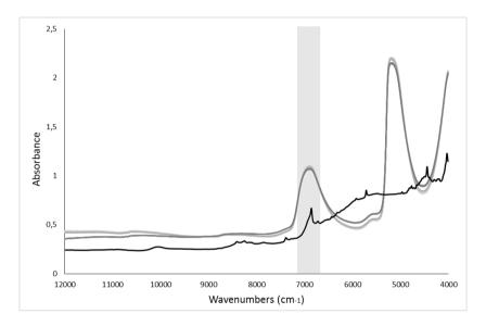
Figure 3: spectra of the acerola juice added with increasing amount of vitamin C (in grey) and spectrum of the ascorbic acid powder (in black). The selected wavelengths are highlighted in grey.
