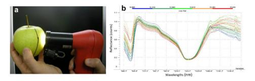
Figure 3: *a* Detail of the probe of the automatic bench-top VIS-NIR system and *b* example of spectra in the 600–1200 nm range (different colors correspond to different TSS values)
