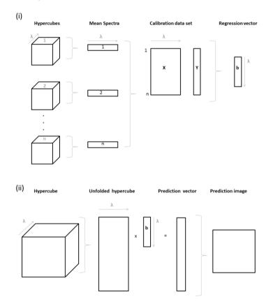
Figure 13. Application of regression modelling to hyperspectral images ('hypercubes'). (i): calculation of mean spectra from sample images and construction of regression vector (b), (ii): application of regression model to hypercube, resulting in prediction image.
