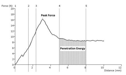
Figure 1: Force-distance curve obtained from the penetration test and
