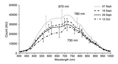
Figure 3: Average raw spectra of 1,360 berries grouped in four sampling dates corresponding to the final stages of ripening.
