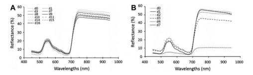
Figure 4: Example of average spectra of Valerianella leaf samples grouped for sampling day (from d0 to d16) for samples stored at 10 C (A) and from d0 to d7 for samples stored
