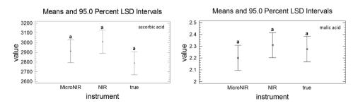
Figure 4: Duncan test on the ANOVA results between the two instruments and the chemical data
