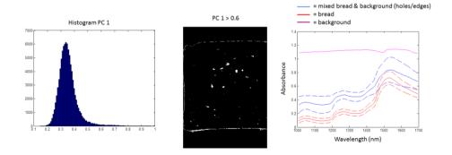
Figure 6. Principal component (PC) score images for a bread sample. Histogram of PC 1 is used to identify mixed edge pixels and holes in the bread. Spectra of bread, background and mixed pixels also shown.
