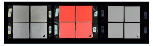
Figure 1: specimens at day 7 – a "steel" b "plastic" c "ceramic" with clean specimens at the top (TQ and Br) and contaminated specimens at the bottom (M1 and M2).
