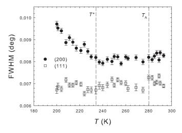
FIG. 6. Temperature evolution of the (200) and (111) Bragg families FWHM for the cubic phase of  $EuTiO_3$ .
