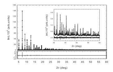
FIG. 3. Measured (dots) and calculated (lines) powder-diffraction patterns for  $EuTiO_3$  at 100 K. The inset shows a magnified view of the high-angle diffraction peaks. The difference between the observed and fitted patterns is displayed at the bottom of each figure.
