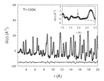
FIG. 7. Observed (dots) and calculated (continuous line) PDF obtained for EuTiO<sub>3</sub> at 100 K. The residual plot is shown at the bottom of the figure. In the inset, a region of short interatomic distances is displayed. The dashed line is the baseline and corresponds to  $-4\pi r\rho_0$  [see Eq. (1)]. The arrow indicates approximately the *r* position of Ti-O interatomic distances.
