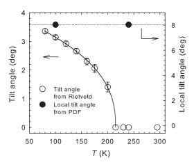
FIG. 5. EuTiO<sub>3</sub> octahedral tilting angle values (empty circles) as a function of temperature obtained from the Rietveld refinement (Table I). The continuous line is the best fit for the critical equation  $\phi_{-}(T) = \phi_{-}(0)(1 - T/T_c)^{\beta}$ , by setting  $T_c = 215$  K. The full circles are the tilting angle values obtained from PDF refinements (Table II).
