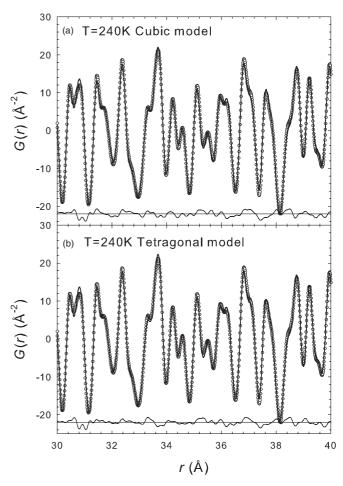
FIG. 8. Short-range observed (dots) and calculated (continuous lines) PDF for  $EuTiO_3$  at 240 K. (a) and (b) are the fits obtained using the cubic *average* model and the low-temperature tetragonal model, respectively. The symbols in the panel label the PDF peaks belonging to Eu-O (stars), Eu-Eu (empty squares), and Ti-O (full circles) interatomic distances.
