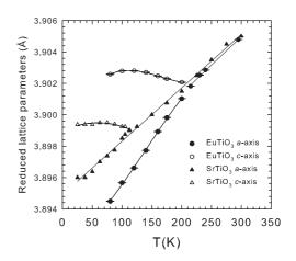
FIG. 2. Reduced lattice parameters of  $EuTiO_3$  and  $SrTiO_3$  as a function of temperature. The full and opened circles are the *a* and *c* axes of  $EuTiO_3$ . Full and opened triangles indicate the *a*- and *c*-axis values of  $SrTiO_3$  derived from Ref. 21. The continuous lines are guides to the eye.
