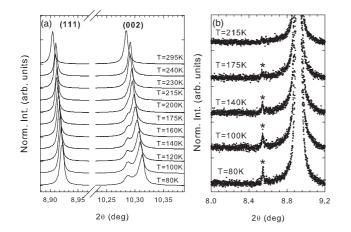
FIG. 1. Selected  $2\theta$  regions of EuTiO<sub>3</sub> x-ray diffraction patterns are shown as a function of temperature. (a) The temperature evolution of the Miller index (111) and (002) peaks related to the room-temperature cubic phase. (b) The appearance of a weak superlattice reflection as a function of temperature.
