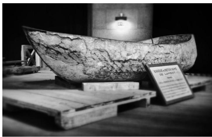
**Fig. 2.4:** Lambot's reinforced cement boat (1848).
