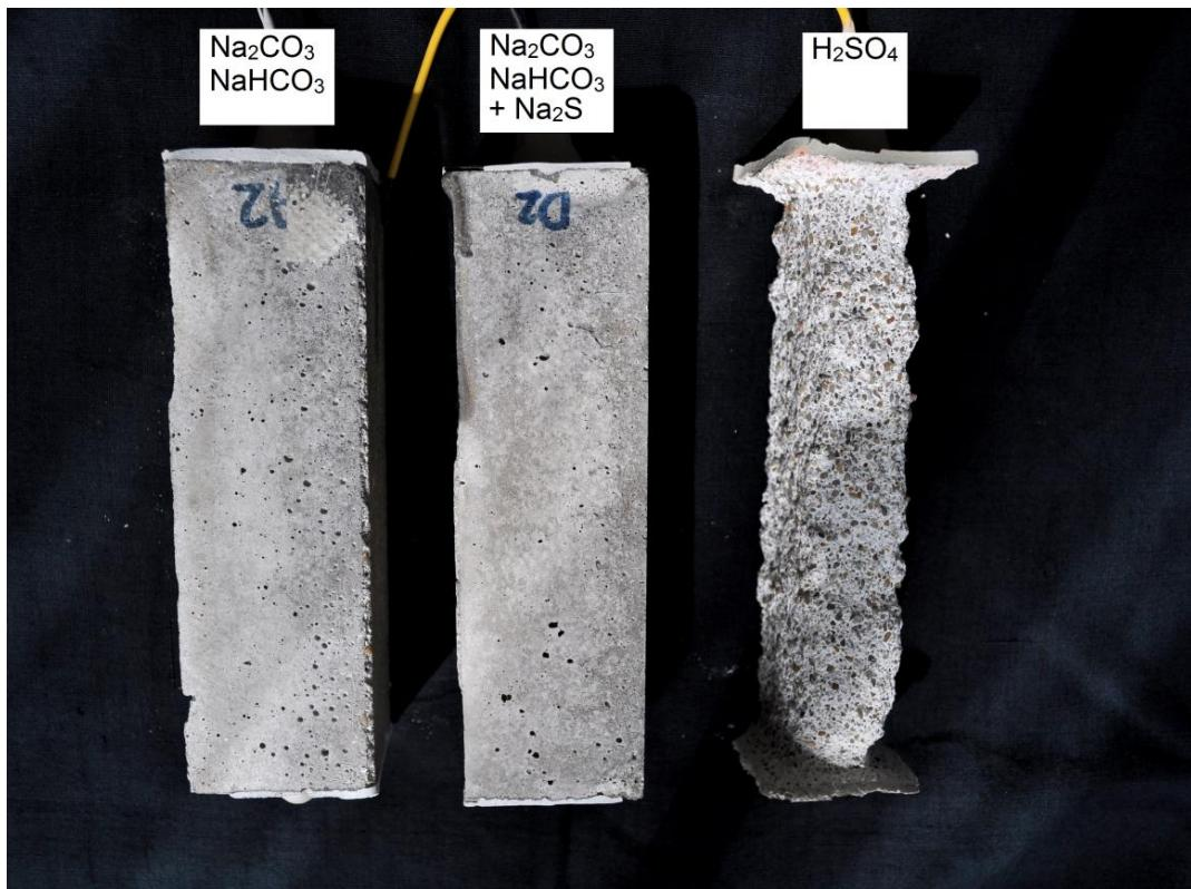
**Fig. 4.33:** Picture of reinforced mortar samples after a 500 days conditioning in three different solutions.
