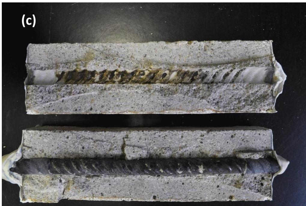
**Fig. 4.32:** Pictures of split reinforced mortar samples after a 200 days conditioning in three different solutions : (a)  $\text{Na}_2\text{CO}_3 / \text{NaHCO}_3$  pH 9, (b)  $\text{Na}_2\text{CO}_3 / \text{NaHCO}_3$  pH 9 +  $\text{Na}_2\text{S}$  2 mM, (c) 0.5%  $\text{H}_2\text{SO}_4$ .
