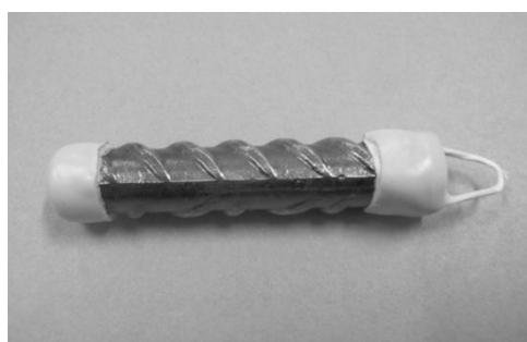
**Fig.4.1:** Steel sample for weigh loss measurements.
