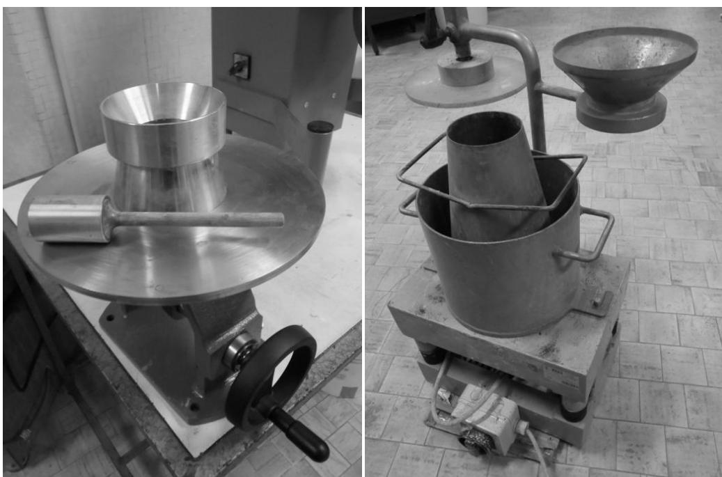
**Fig. 1.3:** Workability testing devices. Left side: flow table (mortar). Right side: Vebe apparatus (concrete).
