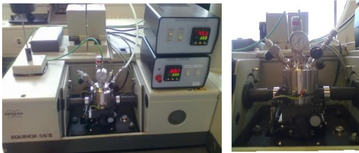
Figure 5.4 Homemade batch-reactor cell
