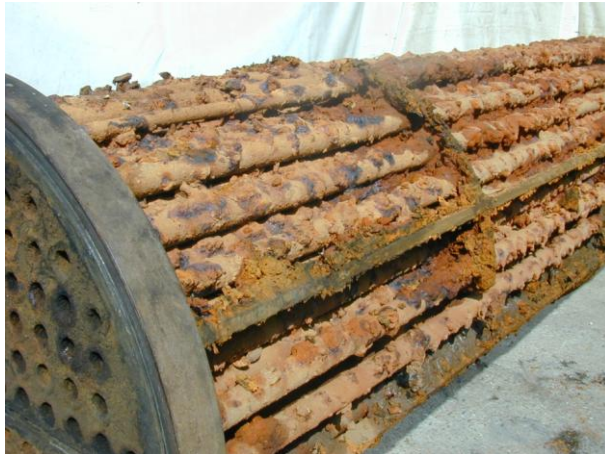
Figure 1-1. Example of crystallization fouling in a shell and tube heat exchanger .
