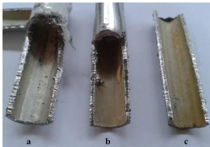
Figure 5-12. Pictures of tubes section after the fouling test (48 hours): Uncoated surface (a); S10 coated surface (b); F10 coated surface (c).
