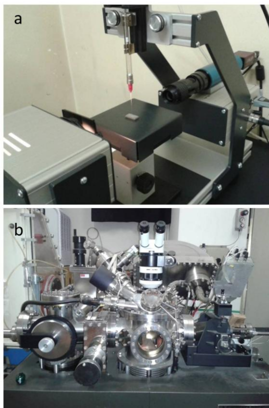
Figure 3-4. Laboratory instrumentation for contact angles measurements (a), and XPS analyses (b).
