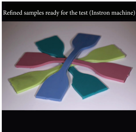
FIGURE 4: Refined dumbbell test specimens ready for the test (Instron machine).
