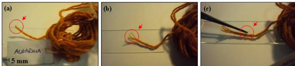
Figure 4. Photographs of (a) the whole thread, (b) a single ply, (c) a single fiber from reference wool (figure from ref. 1).
