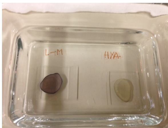
Figure 7. Silver films obtained from 0.1 M colloid of Lee and Meisel (left) and of Leopold and Lendl (right).
