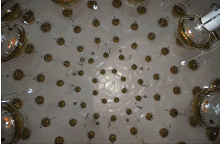
FIGURE 2: Internal view of the LSV neutron veto from its top port.
