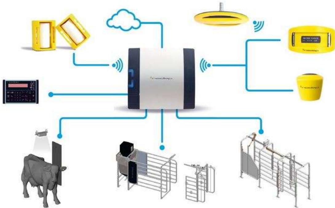
Figure 3 Example of an integrated herd management system based on electronic identification, in which data from different sensors (e.g. pedometers, milk yield recordings, etc.) are collected and processed by a unique platform that controls and manages various aspect of the production process such as individual feeding, separation of sick animals, advices of animals in heat . The entire cycle of the animal can be tracked and managed by and trough this system. In this case data are collected and processed locally, but there is also the option of a cloud-based management. Moreover, the results of data analysis are displayed on PC, smartphone or tablet and the system automatically produces attention alerts about animal in heat or changes in behaviour that may indicate health problems, for example.
