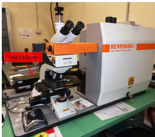
Figure 2.9: Renishaw-Invia system equipped with a 633 nm laser source utilized for micro-Raman spectroscopy.
