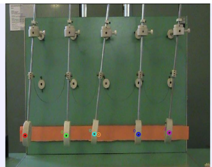
Figure 5.51.: A screenshot of the video of five coupled pendulums
