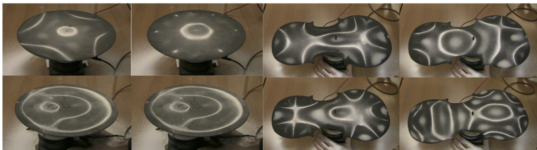
Figure 5.58.: Two dimension systems: the normal modes in Cladni plates.
