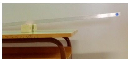
Figure 5.15.: The seesaw on a flat pivot: the scheme (left) and the picture of the real experiment (right). The dot at the very end of the bar is the target to be tracked with Tracker software.
