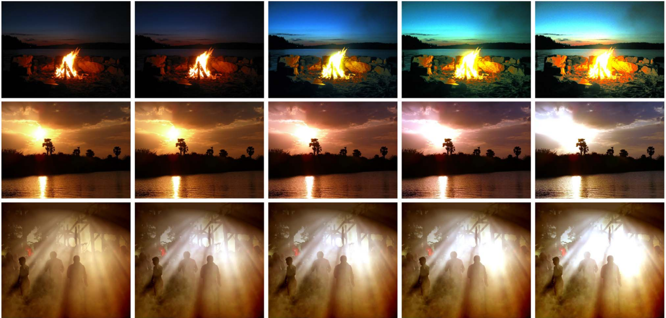
Fig. 3. Comparison among results from different quantile values. The first image of each row is the original; then, from left to right, the QBRIX results using the 99th, 97th, 94th, and 88th quantile as the reference white value.
