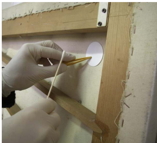
Fig. 4: Sampling by means of nitrocellulose membrane.
