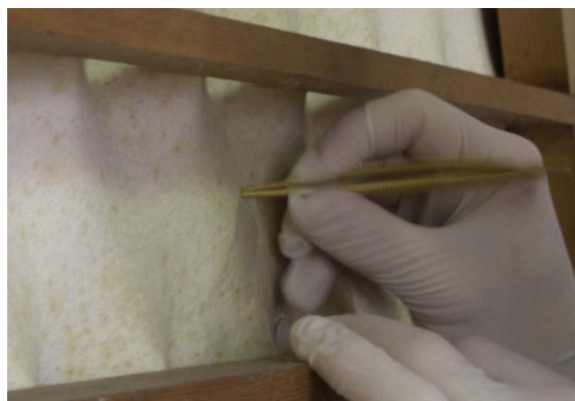
Fig. 5: Sampling by means of fungi-tape.
