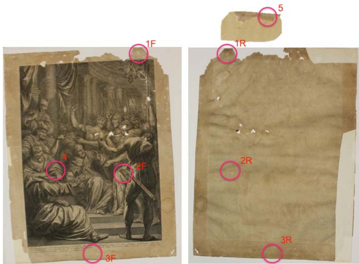
Fig. 2: Localization of the sampling points of Print n°10, indicated in red. Left image: front of the print, right image: back of the print.
