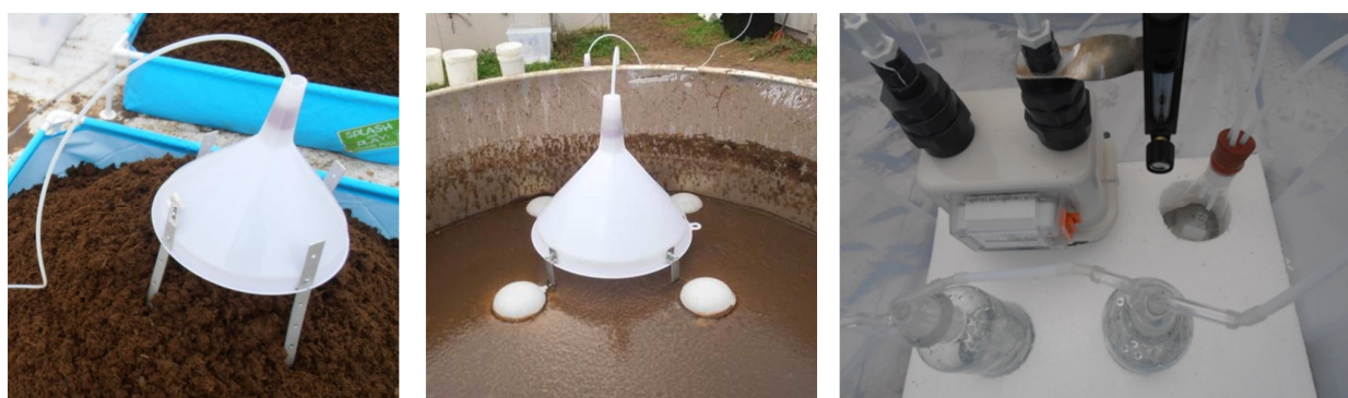
Figure 6 Funnel systems placed on solid fraction (left) and slurry surface (centre) and acid traps (left)
